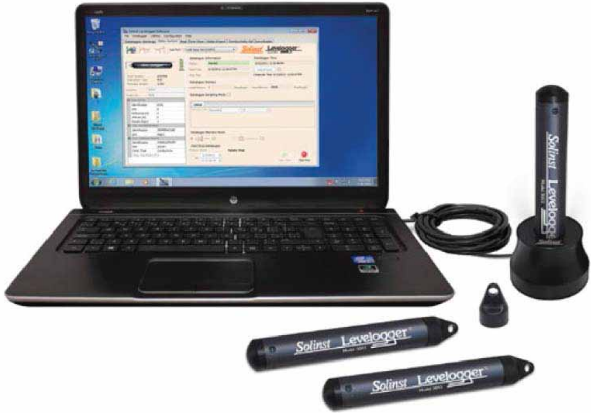
Figure 2-2: Picture of typical pressure Solinst transducer.
