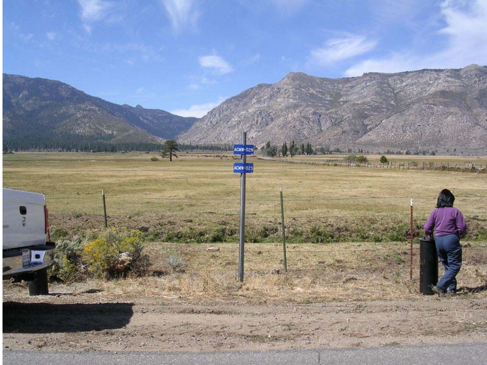
Photo of ACMW-02N and ACMW-02S near the road with no bollards for protection
