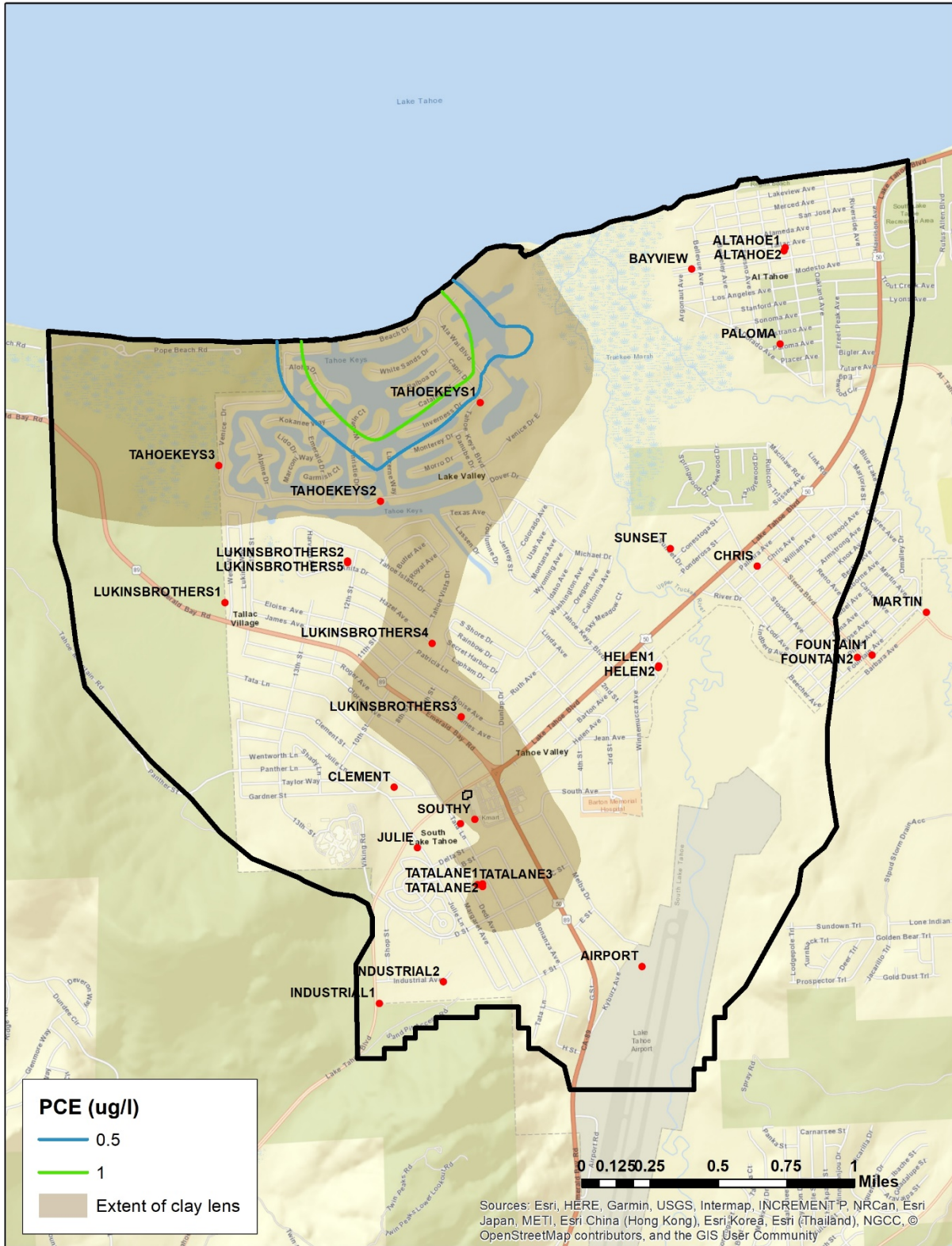
Figure 37. Alternative 1 – Base Treatment. Simulated PCE plume in model layer 2 at the end of the 2068 water year. All concentrations are below the MCL for this stress period.
