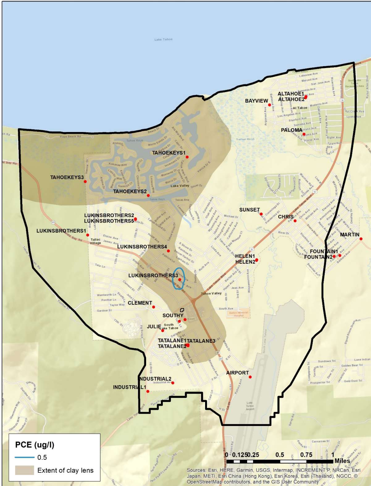
Figure 34. Simulated PCE plume in model layer 4 at the end of the 2018 water year.
