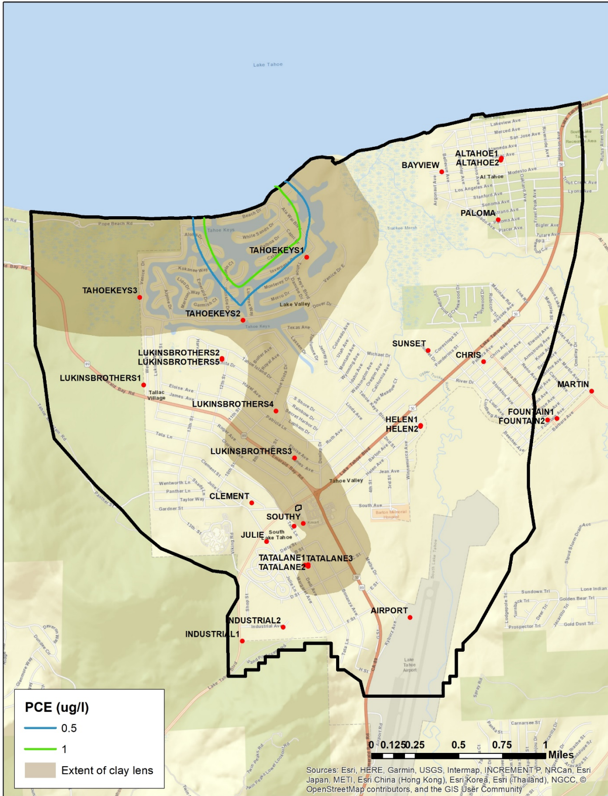
Figure 53. Alternative 2 – Targeted Pumping. Simulated PCE plume in model layer 2 at the end of the 2068 water year. All concentrations are below the MCL for this stress period.
