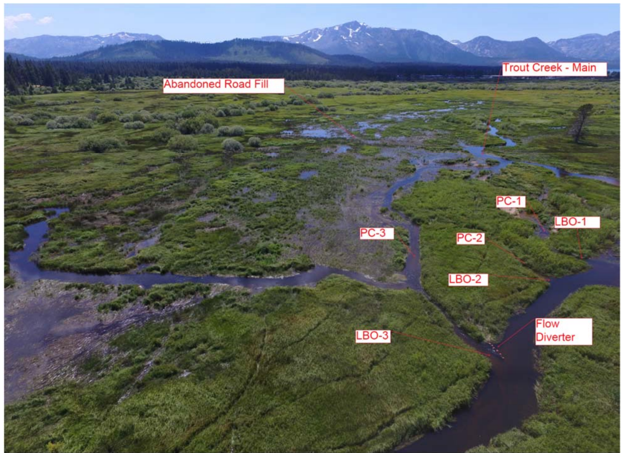
Figure 4-10. Upstream of Bellevue work area looking west, 28 July 2017, with pilot channels diverting flow to left)
