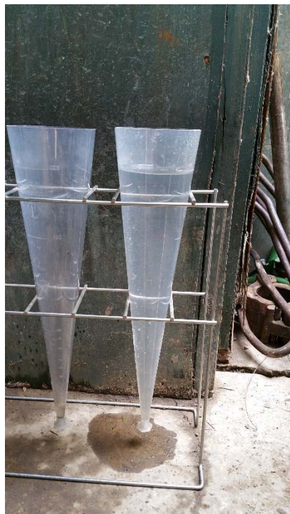
20. 032816 Constant-Rate Imhoff Cones time 1449
