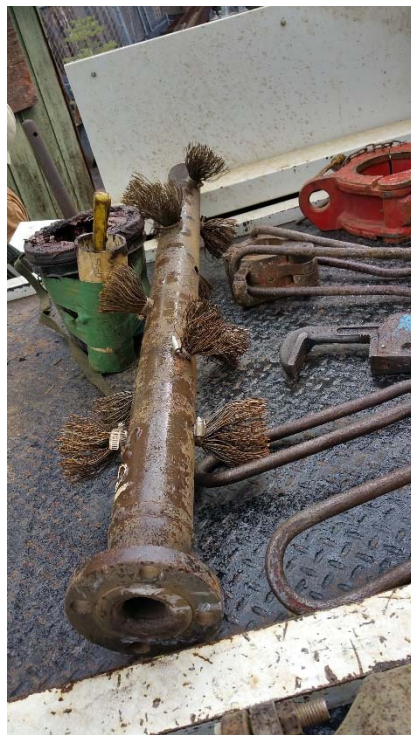
8. Wire brush used for mechanical cleaning
