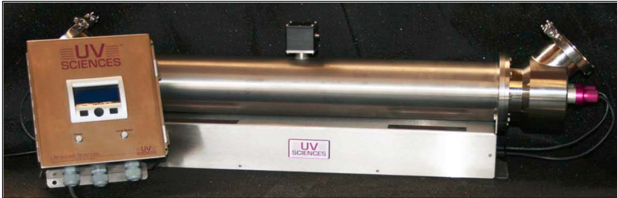
Figure 3-4. NeoTech UV Pilot Test Unit
