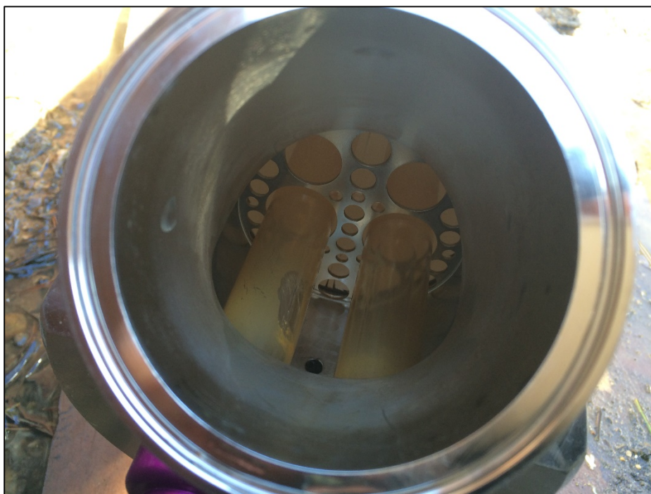
Figure 3-5. Quartz Sleeve Coated with Iron Precipitate
