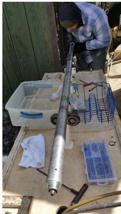
14. Pacific Surveys depth discrete sampling tool
