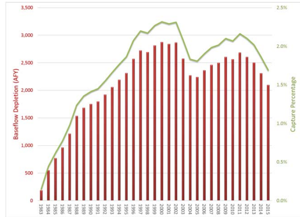
Baseflow depletion for the TVS Basin caused by groundwater pumping. The capture percentage is calculated as the ratio of baseflow depletion and average annual runoff (124,000 acre-ft/yr) (from Pohll et al, 2018)
