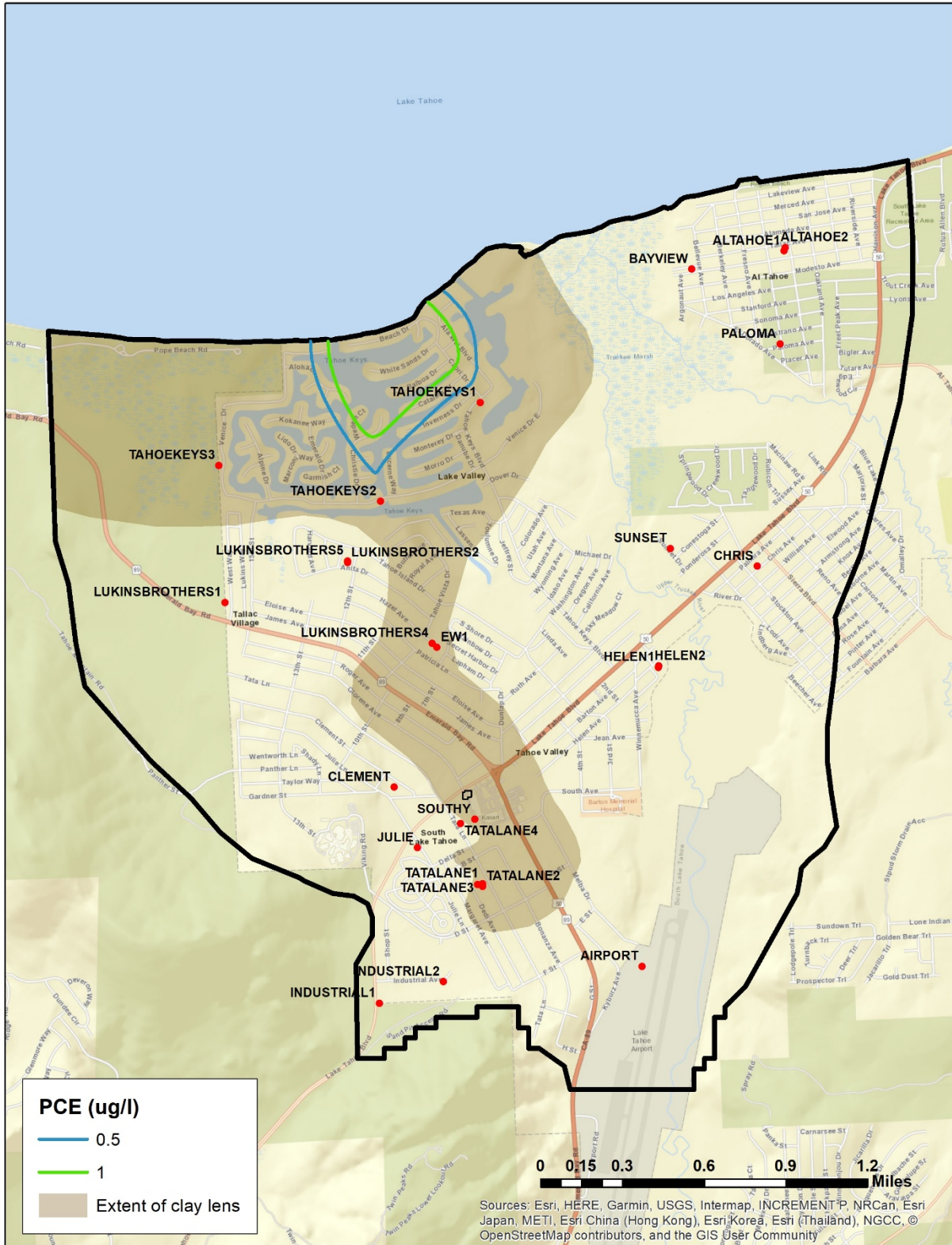
Figure 18. Alternative 2A, Option 2. Simulated PCE plume in model layer 2 at the end of the 2068 water year.
