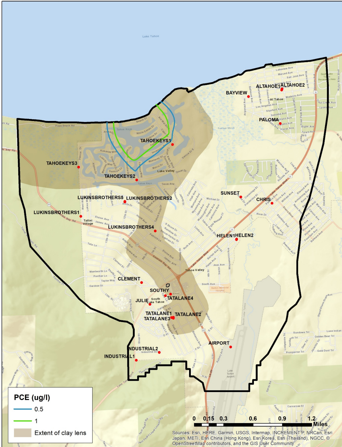
Figure 2. Alternative 2A, Option 1. Simulated PCE plume in model layer 2 at the end of the 2068 water year. All concentrations are below the MCL for this stress period.
