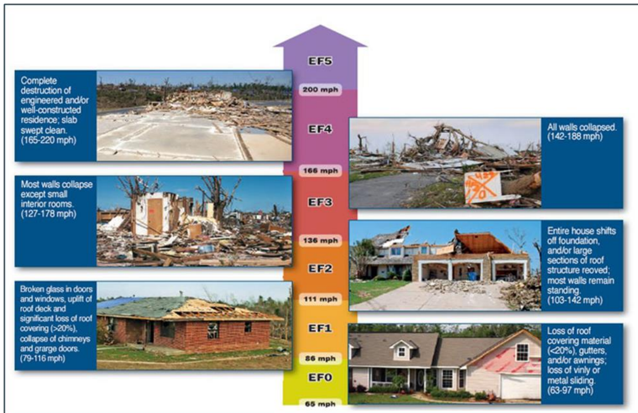
Figure 4-30 Potential Damage Impacts from a Tornado
